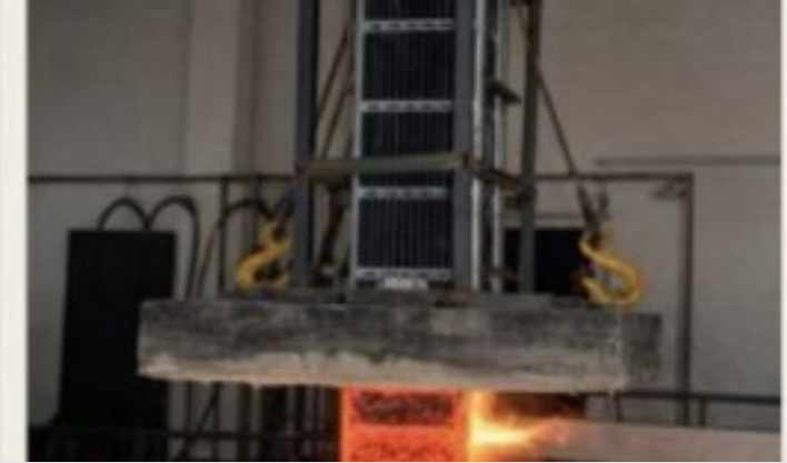
CBRI fire test in progress — furnace, specimen wall
