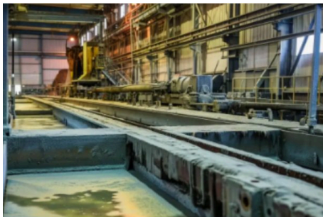
Serangan uap asam — bangsai pickling
